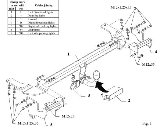
This towbar is designed to assembly in following cars: **MITSUBISHI GRANDIS VAN**, produced since 04.2004, catalogue no. **Z34A** and is prepared to tow trailers max total weight **1800 kg** and max vertical load **85 kg**.
