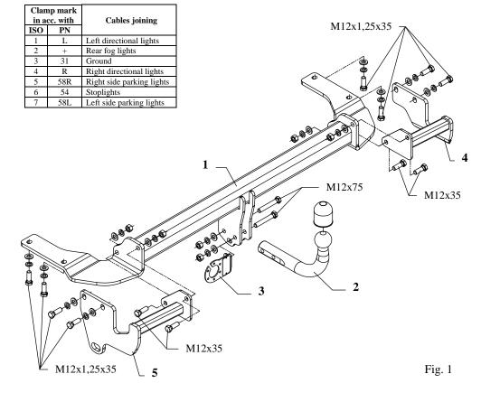
This towbar is designed to assembly in following cars: **MITSUBISHI GRANDIS VAN**, produced since 04.2004, catalogue no. **Z34** and is prepared to tow trailers max total weight **1800 kg** and max vertical load **85 kg**.
