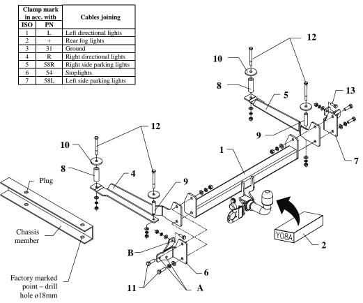
This towbar is designed to assembly in following cars: **HONDA ACCORD 4/5 doors**, (CG, CH), except Coupe, produced since 11.1998 till 10.2002, catalogue no. **Y08A** and is prepared to tow trailers max total weight **1500 kg** and max vertical load **60 kg**.
