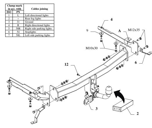
This towbar is designed to assembly in following cars: **DAEWOO NUBIRA II, 4 doors (150),** produced since 07.1999 till 06.2003, catalogue no. **X11A** and is prepared to tow trailers max total weight **1200 kg** and max vertical load **70 kg**.
