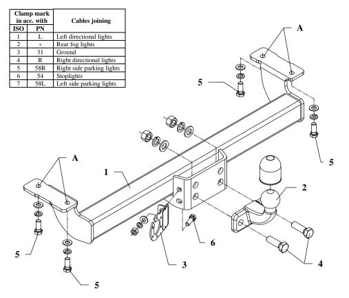
This towing hitch is designed to assembly in following cars: SUZUKI VITARA, 3 door, except V6, spacing of holes in frame 810mm, produced since 10.1988 till 08.1998, catalogue no. W07 and is prepared to tow trailers max total weight 1500 kg and max vertical mass 75 kg.
