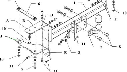
This towing hitch is designed to assembly in following cars: **SUZUKI SAMURAI**, 3/5 doors, only short body cars 3430mm,, produced since 1982, catalogue number **W06** and is prepared to tow trailers max total weight up to 1300 kg and max vertical mass 75 kg.
