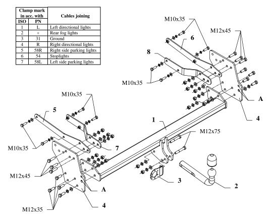
This towing hitch is designed to assembly in following cars: **NISSAN PICK UP/double cabin (240/270) 4x4, tube bumper (D22),** produced since 01.2002 till 06.2005, catalogue no. **V51** and is prepared to tow trailers max total weight **2800 kg** and max vertical load **115 kg**.
