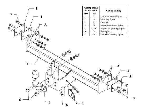
This towing hitch is designed to assembly in following cars: NISSAN TERRANO II, 3/5 doors, (R20), produced since 02.1993 till 02.2005, FORD MAVERICK, 3/5 doors, R20, UDS, UNS, produced since 06.1993 till 04.2001, catalogue no. V18 and is prepared to tow trailers max total weight 3000 kg and max vertical mass 100 kg.
