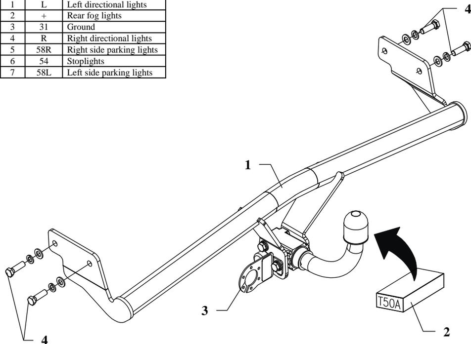
This towbar is designed to assembly in following cars: **KIA RIO II, 5 doors**, produced since 08.2005 till 09.2009, catalogue no. **T50A** and is prepared to tow trailers max total weight **1100 kg** and max vertical load **50 kg**.
