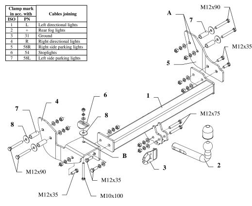
This towing hitch is designed to assembly in following cars: **KIA SPORTAGE, 5 doors, 2/4WD (JA),** produced since 04.1994 till 09.2004, catalogue no. **T10** and is prepared to tow trailers max total weight **2000 kg** and max vertical load **75 kg**.
