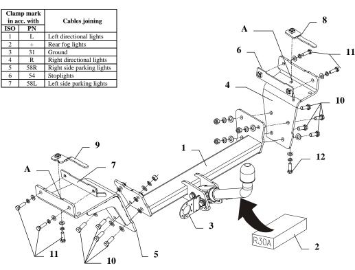
This towbar is designed to assembly in following cars: **FIAT STILO 3/5 doors, except Abarth,** produced since 10.2001 till 03.2007, catalogue no. **R30A** and is prepared to tow trailers max total weight **1400 kg** and max vertical load **60 kg**.
