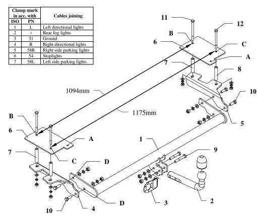
This towing hitch is designed to assembly in following cars: **FIAT PALIO WEEKEND ESTATE (178)**, produced since 01.1998 till 10.2003, catalogue no. **R15** and is prepared to tow trailers max total weight **1200 kg** and max vertical mass **70 kg**.
