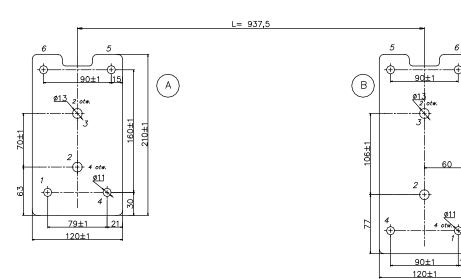
Figure 2. Fish-plates placement
