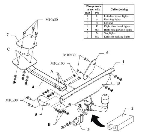
This towbar is designed to assembly in following cars: **FIAT PUNTO, 3/5 door (176),** produced since 09.1993 till 08.1999, catalogue no. **R07A** and is prepared to tow trailers max total weight **1300** kg and max vertical load **50** kg.
