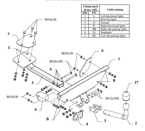
This towbar is designed to assembly in following cars: **FIAT PUNTO**, 3/5 door (176), produced since 09.1993 till 08.1999, catalogue no. **R07** and is prepared to tow trailers max total weight 1300 kg and max vertical load 50 kg.
