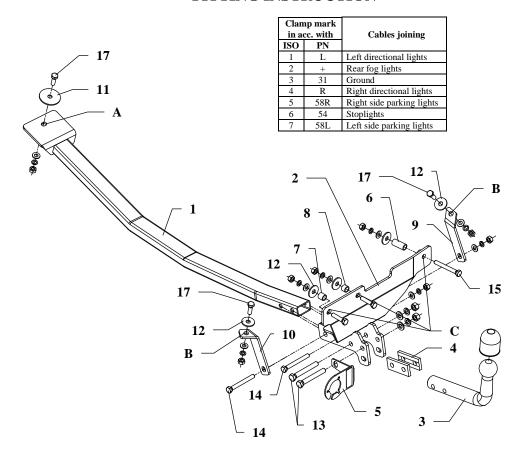
This towing hitch is designed to assembly in following cars: **FIAT TIPO, 3/5 doors,** produced since 06.1988 till 04.1995, catalogue no. **R03** and is prepared to tow trailers max total weight up to **1200 kg** and max vertical mass **75 kg**.
