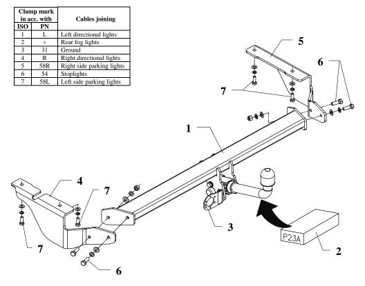
This towbar is designed to assembly in following cars: CITROEN C5 Estate (X42) produced since 04.2001 till 09.2004, catalogue number P23A and is prepared to tow trailers max total weight 1600 kg and max vertical load 85 kg.
