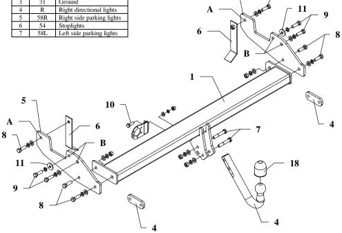
This towbar is designed to assembly in following cars: **TOYOTA HILUX 4WD with double cabin,** produced since 10.2005 till 10.2010, catalogue number **O64** and is prepared to tow trailers max total weight up to **2500 kg** and max vertical mass **100 kg**.
