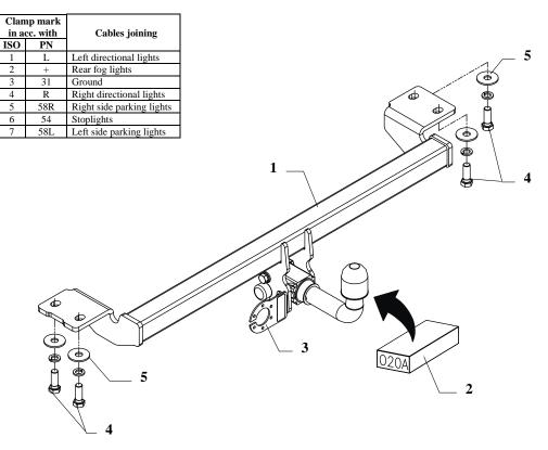
This towbar is designed to assembly in following cars: **TOYOTA AVENSIS ESTATE**, produced since 02.1998 till 03.2003, catalogue no. **O20A** and is prepared to tow trailers max total weight **1575kg** and max vertical mass **75kg**.
