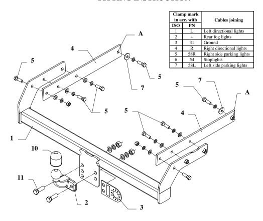
This towing hitch is designed to assembly in following cars: **VOLKSWAGEN T5, loading platform, double cabin,** produced since 04.2003 till 06.2015 and **VOLKSWAGEN T6, loading platform, double cabin,** produced since 07.2015, catalogue no. **K47** and is prepared to tow trailers max total weight **2500 kg** and max vertical load **100 kg**.
