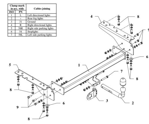
This towing hitch is designed to assembly in following cars: **JEEP CHEROKEE (XJ)**, produced since 02.1997 till 08.2001, catalogue no. **JP01** and is prepared to tow trailers max total weight up to **3300 kg** and max vertical load **100 kg**.
