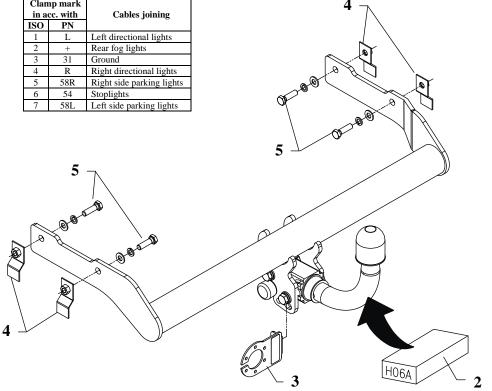
This towbar is designed to assembly in following car: SKODA FELICIA ESTATE, produced since 07.1995 till 06.2001, catalogue no. H06A and is prepared to tow trailers max total weight 1200 kg and max vertical load 50 kg.
