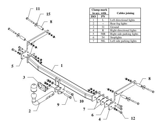
This towing hitch is designed to assembly in following car: **DACIA LOGAN, 4 doors,** produced since 09.2004 till 06.2008 and since 07.2008 till 12.2012, catalogue number **G47** and is prepared to tow trailers max total weight **1100 kg** and max vertical load **75 kg**.
