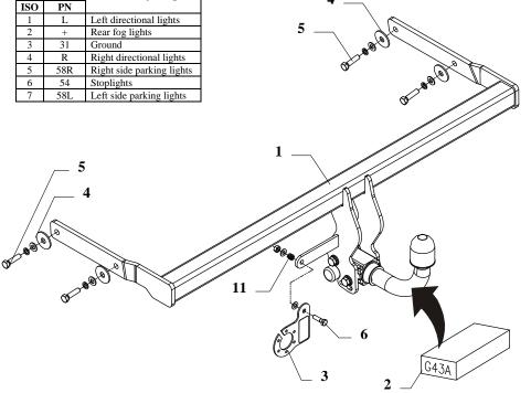
This towbar is designed to assembly in following car: **RENAULT MEGANE II, 4 doors,** produced since 09.2003, catalogue no. **G43A**
