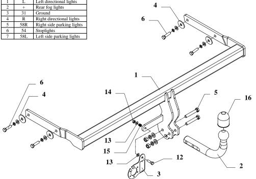
This towbar is designed to assembly in following car: RENAULT MEGANE II, 4 doors, produced since 09.2003, catalogue no. G43 and is prepared to tow trailers max total weight 1300 kg and max vertical load 75 kg.
