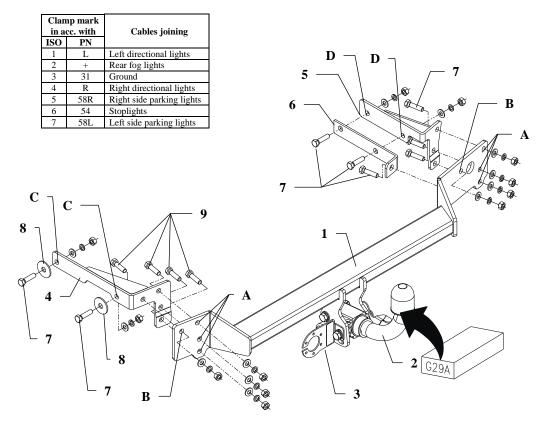
This towbar is designed to assembly in following car: **RENAULT CLIO II/CAMPUS, 3/5 doors, except Sport V6,** produced since 03.1998 till 06.2001 and produced since 07.2001 till 08.2005, catalogue no. **G29A** and is prepared to tow trailers max total weight **1200 kg** and max vertical mass **75 kg**.
