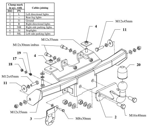
This towing hitch is designed to assembly in following car: **RENAULT ESPACE/GRAND ESPACE, 5 doors, VAN, (JE, J66)** produced since 11.1996 till 09.2002, catalogue no. **G26** and is prepared to tow trailers max total weight **1900 kg** and max vertical load **85 kg**.
