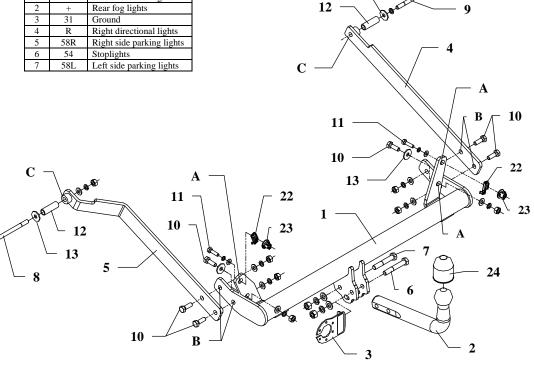
This towing hitch is designed to assembly in following car: **RENAULT MEGANE I CLASSIC, 4 doors, produced since 09.1996 till** 08.2003, catalogue no. G22 and is prepared to tow trailers max total weight 1300 kg and max vertical load 75 kg.
