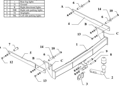
This towing hitch is designed to assembly in following cars: RENAULT SAFRANE, 5 doors, produced since 04.1992 till 12.2001, catalogue no. G20 and is prepared to tow trailers max total weight 1600 kg and max vertical mass 75 kg.
