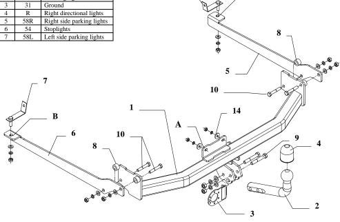
This towbar is designed to assembly in following cars: **PEUGEOT 306 4 door, except Cabrio,** produced since 10.1994 till 05.2001, catalogue no. **F09** and is prepared to tow trailers max total weight **1400 kg** and max vertical load **52 kg**.
