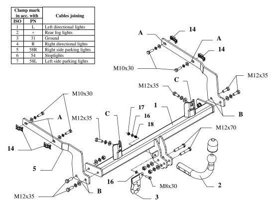
This towing hitch is designed to assembly in following cars: **PEUGEOT 406 BREAK / SW (ESTATE), type D8 and D9,** produced since 01.1997 till 05.2004, catalogue no. **F08** and is prepared to tow trailers max total weight **1700 kg** and max vertical load **80 kg**.
