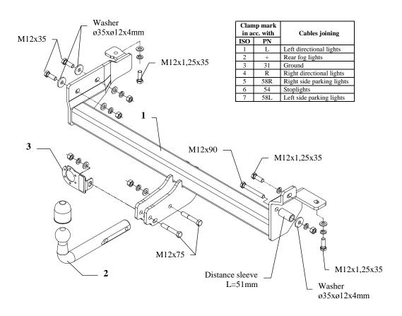
This towbar is designed to assembly in following cars: **OPEL FRONTERA**, **2/4 doors Sport (UT2/UT4)**, produced since 10.1998 till 08.2003, catalogue no. **E44** and is prepared to tow trailers max total weight **2800 kg** and max vertical load **112 kg**.
