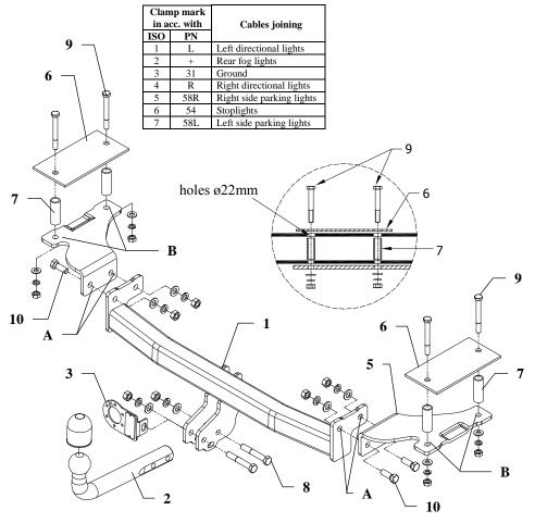
This towing hitch is designed to assembly in following car: **OPEL COMBO (B), passenger car, delivery truck,** produced since 08.1994 till 02.2002, catalogue number **E20** and is prepared to tow trailers max total weight **1200 kg** and max vertical load **50 kg**.
