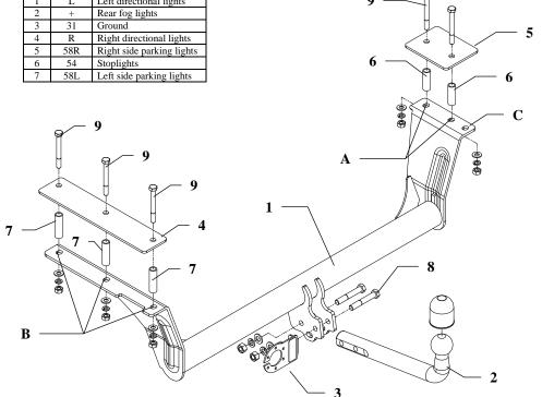
This towing hitch is designed to assembly in following cars: OPEL OMEGA "A" CARAVAN, ESTATE, produced since 09.1986 till 03.1994, catalogue no. E15 and is prepared to tow trailers max total weight 2000 kg and max vertical load 75 kg.
