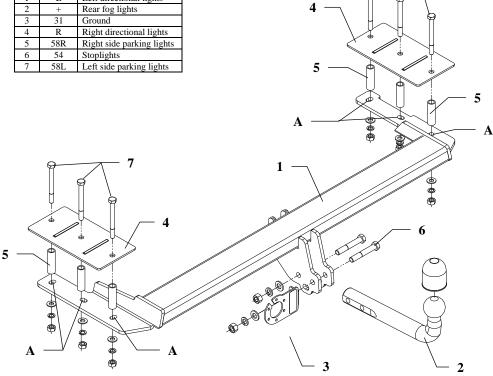
This towing hitch is designed to assembly in following car: OPEL VECTRA (A), 4 doors, except 4x4, produced since 09.1988 till 08.1995, catalogue no. E11 and is prepared to tow trailers max total weight 1700 kg and max vertical load 75 kg.
