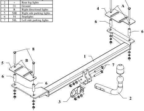
This towing hitch is designed to assembly in following cars: OPEL VECTRA (A), 5 doors, produced since 09.1988 till 08.1995, catalogue no. E011 and is prepared to tow trailers max total weight 1700 kg and max vertical load 75 kg.
