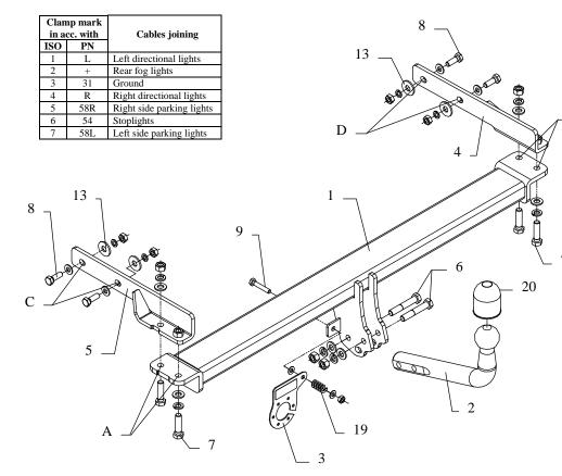
This towing hitch is designed to assembly in following cars: MERCEDES CLASS E, ESTATE (S210), except AMG produced since 05.1996 till 02.2003, catalogue no. D31 and is prepared to tow trailers max total weight 2300 kg and max vertical load 90 kg.
