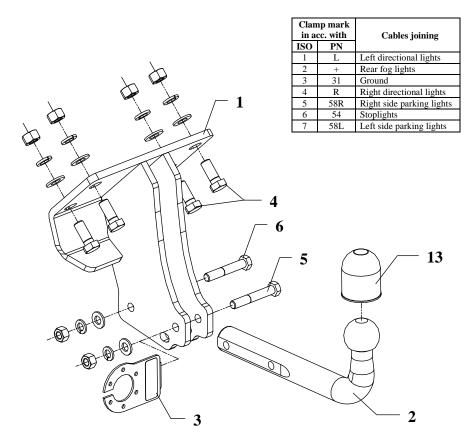
This towing hitch is designed to assembly in following cars: **MERCEDES G-Class**, (W461, W463) produced since 12.1989, catalogue no. **D25** and is prepared to tow trailers max total weight 3500 kg and max vertical mass 120 kg.
