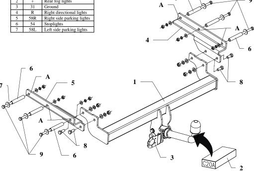
This towbar is designed to assembly in following car: FORD MONDEO Turnier, ESTATE (Mk2), except ST 200 and RS, produced since 09. 1996 till 12.2000, catalogue no. C20A and is prepared to tow trailers max total weight 1800 kg and max vertical load 75 kg.
