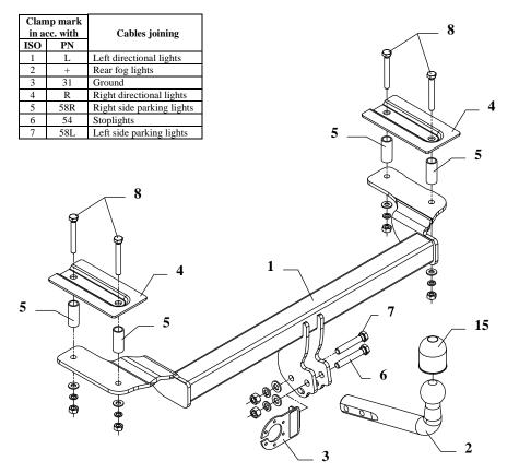
This towbar is designed to assembly in following cars: **FORD FIESTA, 3-5 doors** and **MAZDA 121 JASM/JBSM, 3 doors,** both produced since 02.1996 till 12.2001, catalogue no. **C002** and is prepared to tow trailers max total weight **950 kg** and max vertical load **50 kg**.
