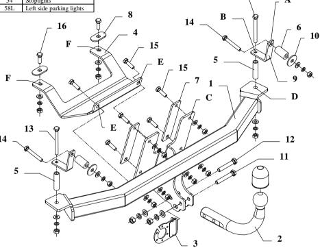
This towing hitch is designed to assembly in following car: **ALFA ROMEO 146,** produced since 1995 till 2001, catalogue no. **AL32** and is prepared to tow trailers max total weight **1300 kg** and max vertical load **75 kg**.
