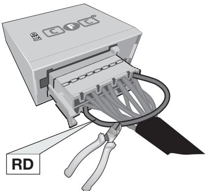
Pin 11 and Pin 2 disconnected
